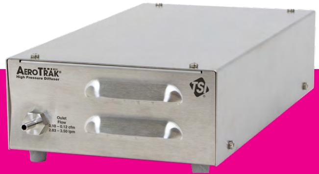
The TSI AeroTrak® High Pressure Diffuser (HPD) Model 7950 accessory allows the TSI AeroTrak Particle Counters to measure particulate contamination in high-pressure compressed gas systems. As particle counters cannot sample high pressure gas, they require HPD accessories to reduce the pressure of compressed gases to assess the cleanliness level of compressed gas systems.
